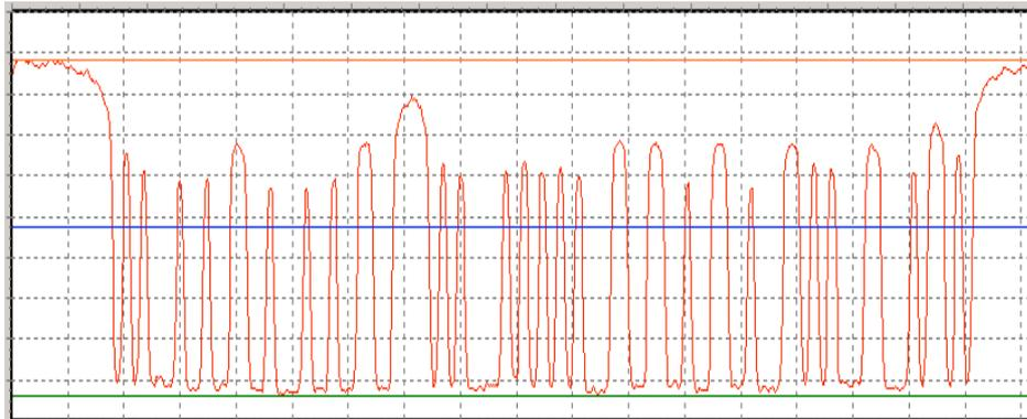
If there is too much ink spread, the narrow spaces will become even narrower and not appear as white as other wider spaces in the bar code. This means that there will be lower minimum edge contrast, while symbol contrast remains the same. Modulation is measured by comparing the edge contrast minimum to the symbol contrast.
