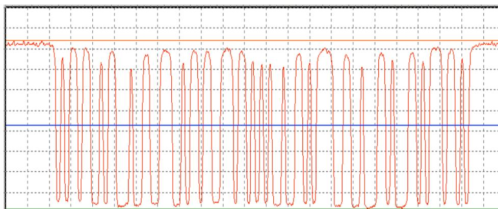
This graph shows the reflectance of the darkest bar with the horizontal green line, the reflectance of the palest spaces (in this example, the quiet zones) with the horizontal orange line, and the halfway point (the global threshold) is shown by the horizontal blue line.
