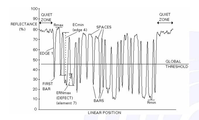
For each scan the verifier produces an individual reflectance profile which measures the reflectance of each bar and space of the bar code. The verifier then takes nine different measurements from the reflectance profile, and grades seven of them individually.
